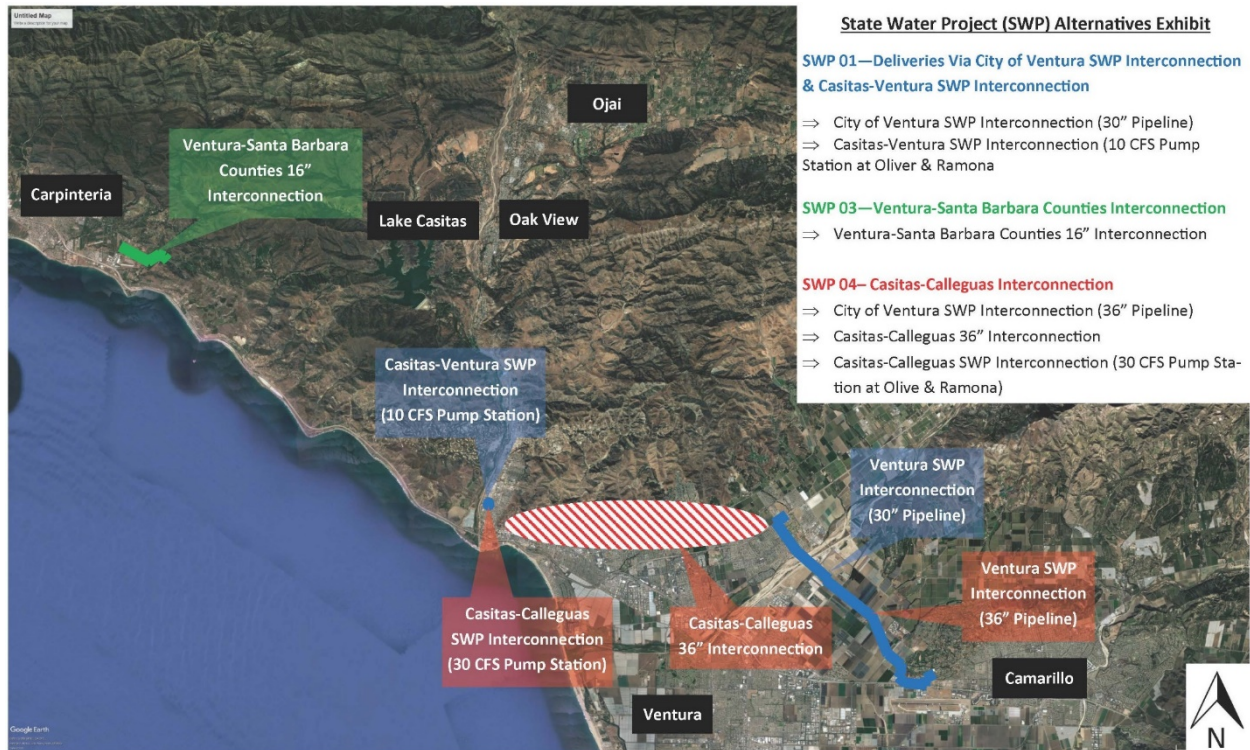
Figure 5-10 Casitas State Water Project Interconnection Options
